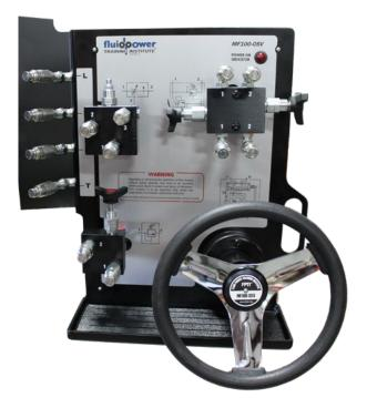
Every component on the "TS" model is equipped with FPTI™'s exclusive auto-fault technology, which simply means every component can be made to "wear out" in real-time. No need to exchange cartridges.
